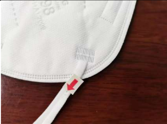
87_defect-Dirt mark at loop-mi
