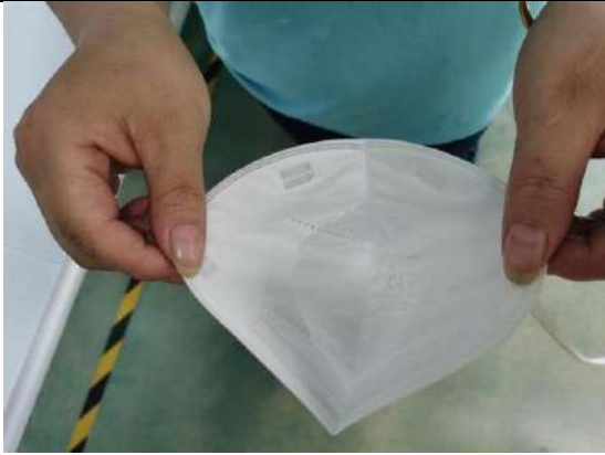
73_Water penetration check check of filter
