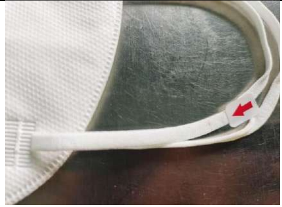
86_defect-Dirt mark at loop-mi
