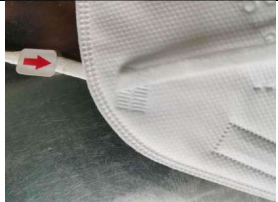
88_defect-Dirt mark at loop-mi
